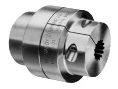
The Clamp-Type Coupling utilized the basic Magnaloy coupling with the addition of the clamp feature. Developed to compensate for variations in spline formation methods and tolerances. Assures centering of the coupling and positive retention on the shaft. The clamp feature is suggested for all splined couplings, but is also available in smooth bored and keyed models.
