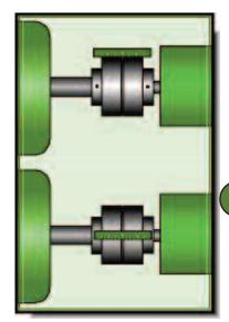
Perfect alignment of equipment shafts, in most cases, is impractical to obtain or maintain, and misaligned equipment produces, excess stress on bearings and the coupling. Magnaloy's insert design will accept misalignment strain and, when excessive, will cause insert wear as a visual and audible indication of misalignment problems. However, Magnaloy's inserts are inexpensive and easily replaces; under normal conditions the insert seldom requires replacement.
