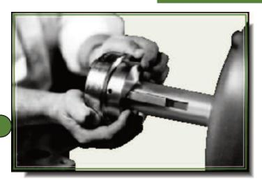
**Shaft spacing** should be within range given by dimensions 'W' and 'X' as shown in charts on page 4.
