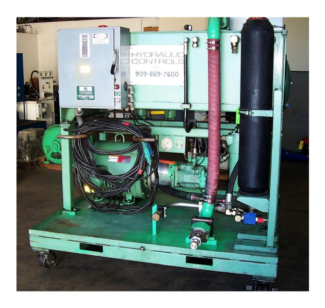
**100 HP Electric**, 460vac, 300-gallon reservoir, 10-gallon Accumulator, 10 micron filter, 56gpm @ 3000psi, Variable pump, motor starter with cables, and remote Estop.
