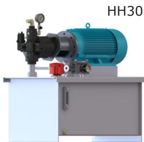
THIS HCI BUILT CUSTOM POWER UNIT COMES WITH AN IN-TANK 10 $\mu$  FILTER, SIGHT / TEMP GAUGE, PRESSURE GAUGE WITH SNUBBER, 3 $\mu$  TANK BREATHER AND A BOSCH REXROTH A10V-SO28 VARIABLE DISPLACEMENT PISTON PUMP COUPLED TO A 10 HP NEMA PREMIUM EFFICIENCY ELECTRIC MOTOR.
