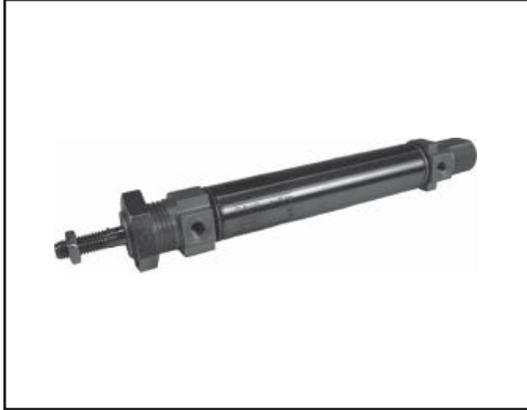
The Series MNI mini-ISO cylinder conforms to ISO 6432, ensuring interchangeability between manufacturers who conform to the same standard. With stainless steel rod and barrel, anodized aluminum end covers, brass piston and Buna-N seals, it provides a rugged construction ensuring years of trouble-free operation. Included in Quick Ship are bore sizes range from 16mm to 25mm, with strokes 10mm, 25mm, 50mm, 80mm, 100mm and 160mm. A comprehensive array of a mounts and rod accessories are available.
