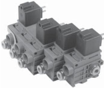
The 3/2 function Series 579 directional control valve with unique poppet design offers trouble free service. Polymer body allows a rugged and corrosion resistant valve. Dove tail design allows combining of valves easily without tools. Integrated pneumatic tube fittings save time and money.
