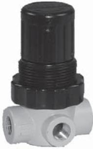
Series MU1 air pressure regulators are 1/8" NPT and 1/4" NPT inch ported units. The compact design and die cast zinc body suits many different applications. Series MU1 are diaphragm type, self relieving, and three pressure ranges are offered in the Quick Ship program.
