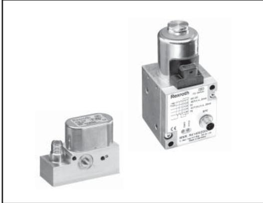
Direct acting poppet style, electro-pneumatic (E/P) pressure control valves with closed loop control. Use to change output pressure or force proportional with an electrical input. Compact ED02 version is only 30mm wide. Also in the Quick Ship program is the higher flow ED05 model.
