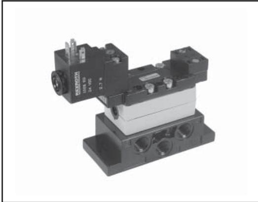
Series 581 directional control valves meet ISO 5599-1 and are interchangeable with many other manufacturers. The 581, in ISO sizes 1, 2 and 3 offers higher flow rates as compared other ISO valves within the same size. Unique spool and sleeve assembly is isolated from vibration and outside forces for long life. Construction allows field convertibility for internal or external pilot control. Valves come with CNOMO operators, coils to be ordered separately. Subbases also ordered separately.
