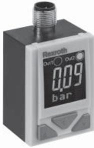
The Series PE5 piezoresistive pressure sensor unit with analog and/or digital outputs can be mounted to NL1, AS2, AS3 or AS5 pressure regulators or distribution blocks, or used stand-alone. They can measure PSI, bar, or kPa. Versions with switching outputs and transducer outputs are available.
